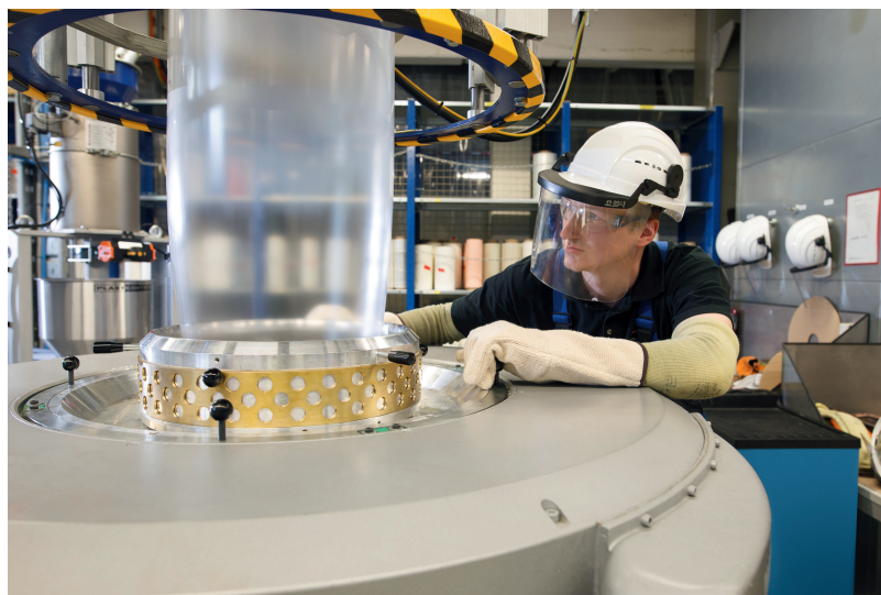
Fig. 1. Covestro blown film line at the Bomlitz site: the plastics manufacturer is currently expanding the production of multi-layer coextruded TPU films there, as demand for them from various industries is increasing. © Covestro
